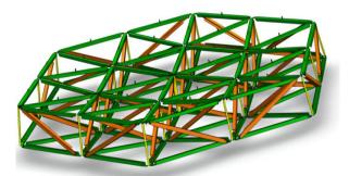
Fig. 1. Support structure of the solar concentrator with triangular mirrors
