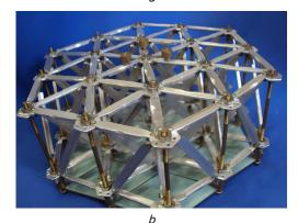
Fig. 2. Structure of the first prototype: a – backside of the concentrator; b – right side of the concentrator with flat triangular mirrors
